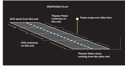
Images above left and left, represent two options for paced collaboration: in the first option (above left), one utility company follows the other with their works (referred to as 'chasing' works); in the second option (left), they approach the road from different sides (referred to as 'spacing' works). Site management and timing must be collaborated to make paced collaboration successful.
